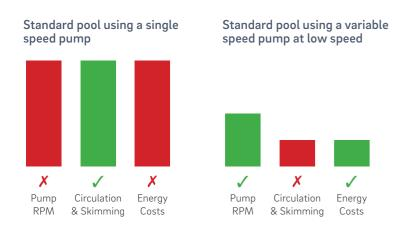
Variable speed pumps are appealing because they present an opportunity to reduce energy costs. Whilst they can turn over a sufficient volume of water at lower pump speeds, skimming power and circulation is compromised. Without sufficient skimming and circulation, water balance is difficult to maintain, algae forms in dead spots and maintenance costs increase significantly.
